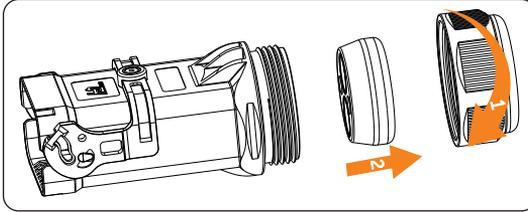
Figure 7-22 Disassembling the AC connector
