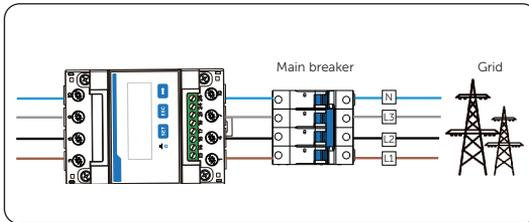
Figure 14-6 Connecting direct-connected meter to the grid
