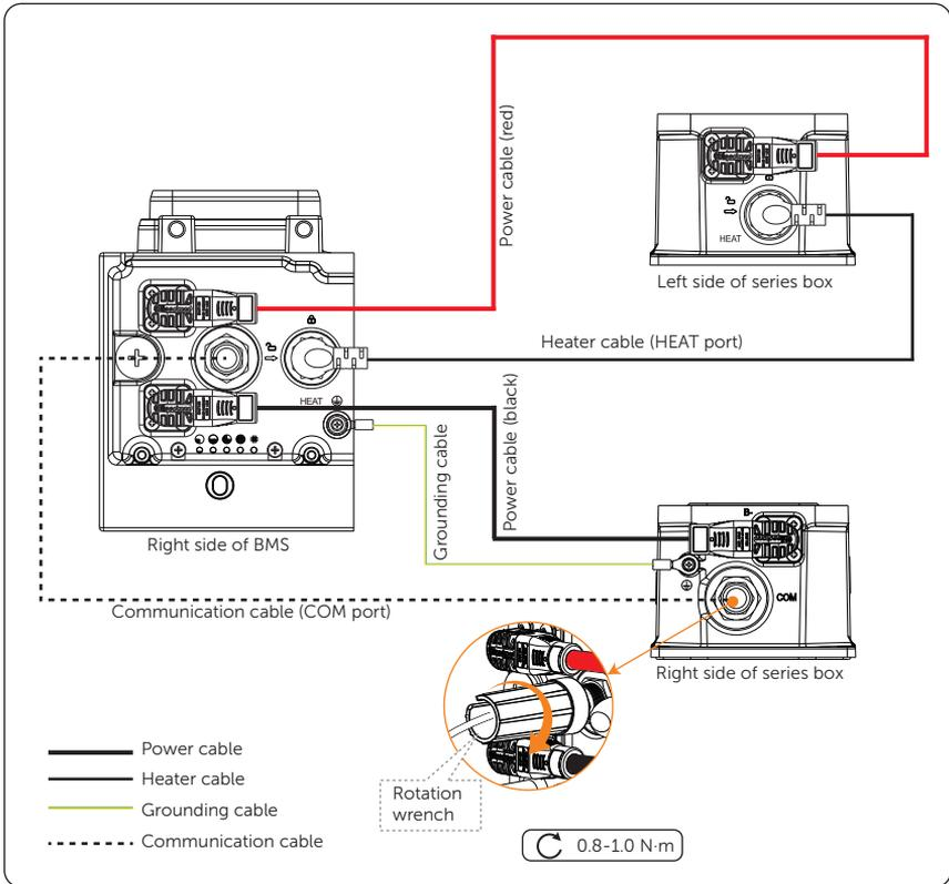
Figure 7-9 Connecting cables
