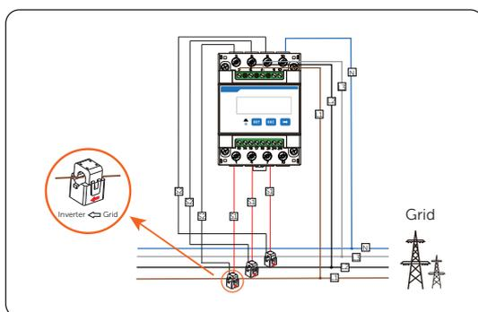
Figure 14-11 Connecting CT-connected meter to the grid
