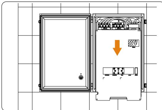
Figure 7-90 Removing the plate
