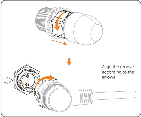
Figure 7-12 Locking heater cable
