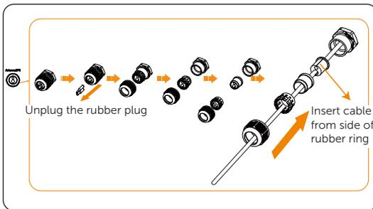
Figure 7-93 Threading the Wi-BR cable through Antenna&PE port
