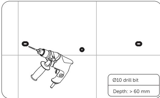
Figure 6-57 Drilling holes
