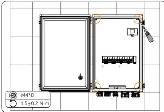
Figure 7-89 Loosening screws on the plate
