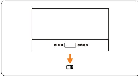
Figure 6-50 Removing the dustproof cover
