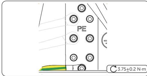
Figure 7-117 Threading the PE cable through Antenna&PE port
