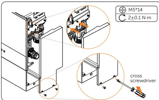
Figure 7-70 Locking the cable shielding board
