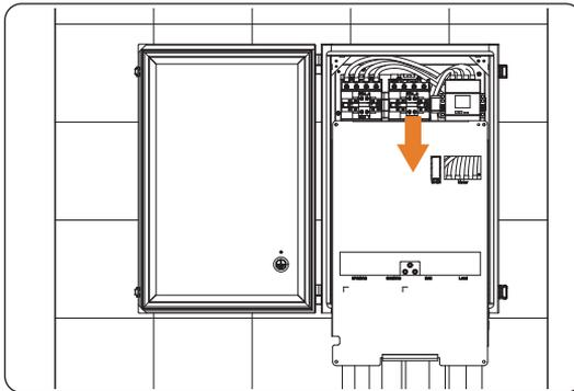
Figure 7-88 Removing the plate
