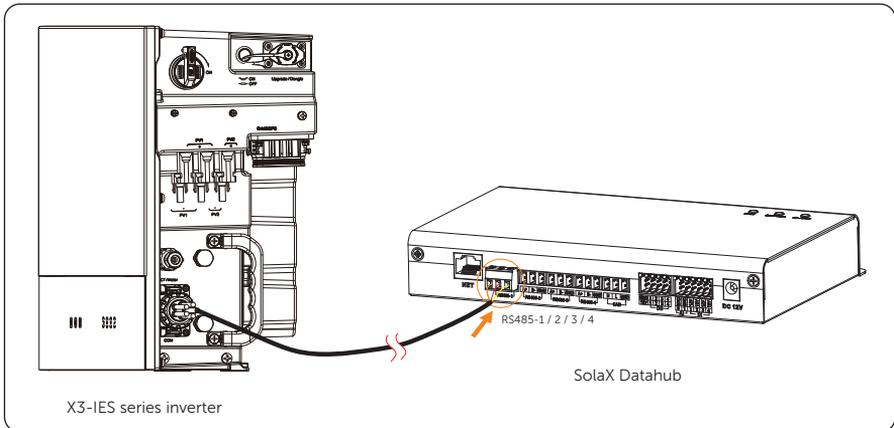
Figure 7-51 Inverter connected with a SolaX databus
