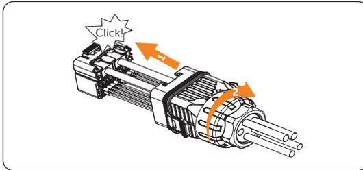
Figure 7-61 Inserting the terminal block into the connector
