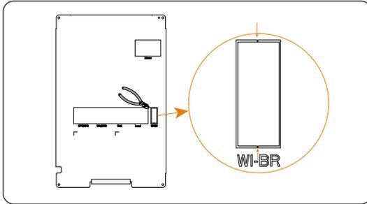
Figure 7-96 Cutting the baffle
