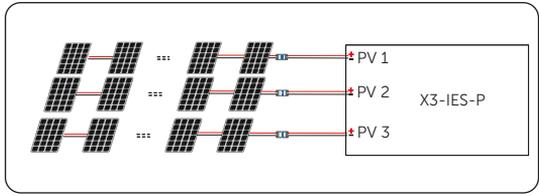
Figure 7-34 "Multi" mode connection diagram for Pro version
