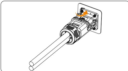
Figure 12-10 Loosening the AC connector
