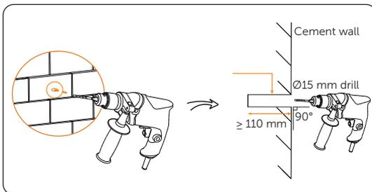
Figure 6-34 Drilling holes
