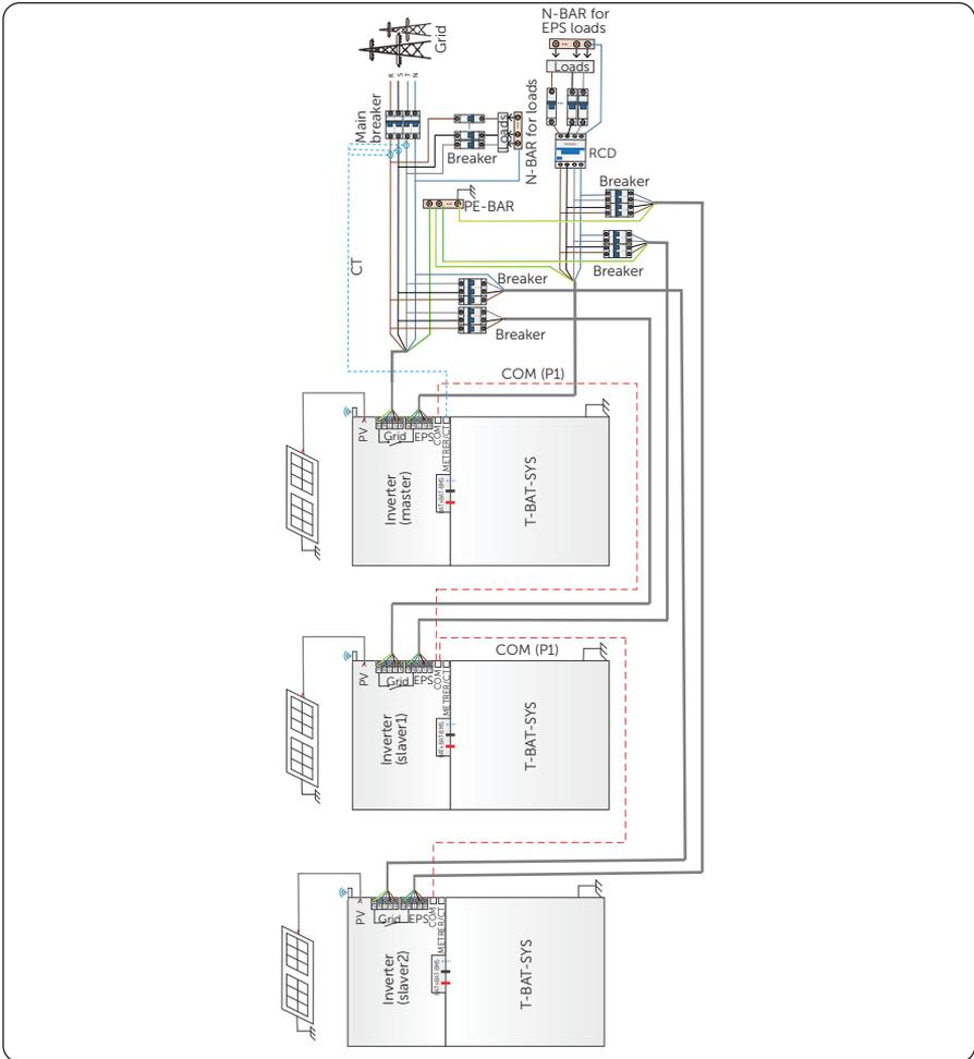
Figure 7-48 System diagram without SolaX X3-PBOX device
