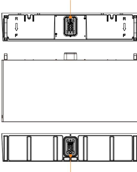
A hot-plug interface that is connected to the bottom of the battery module or the Base.
