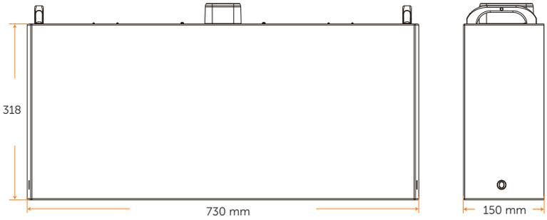
Figure 2-8 Battery module
