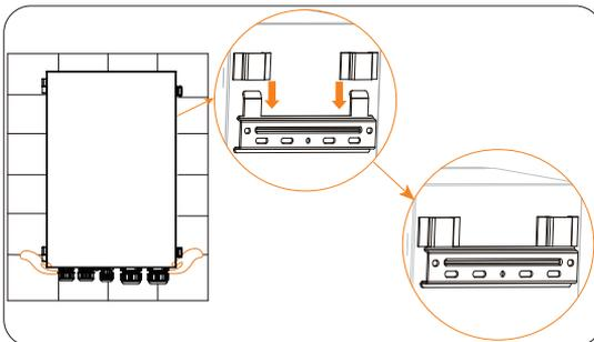
Figure 6-60 Hanging the matebox on the bracket
