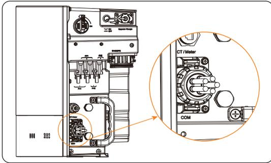
Figure 7-54 Well connected COM port
