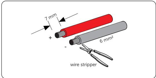
Figure 7-36 Stripping PV cables
