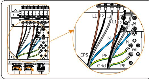
Figure 7-110 Connecting cables to the terminal block in the matebox
