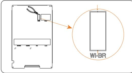
Figure 7-91 Cutting the baffle
