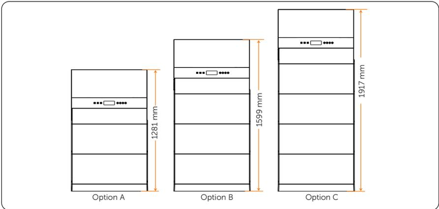
Figure 4-3 Installation options for one tower
