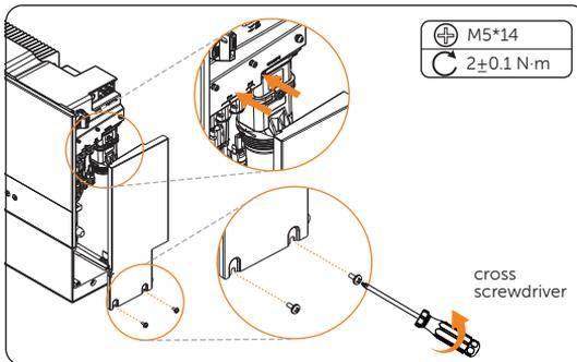
Figure 7-72 Locking the cable shielding board
