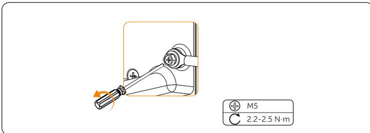
Figure 12-18 Disconnecting grounding cable
