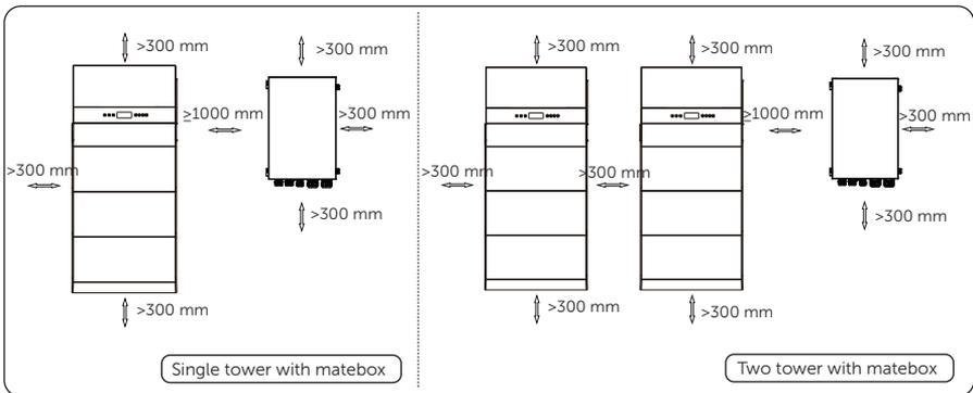
Figure 4-7 Clearance requirement with matebox
