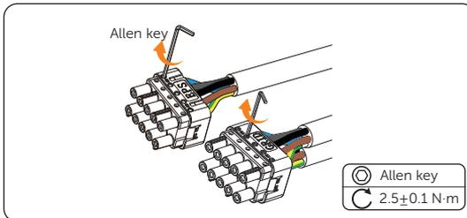
Figure 7-27 Locking wires in the AC connector
