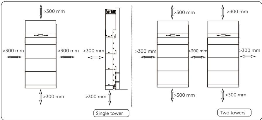
Figure 4-6 Clearance requirement
