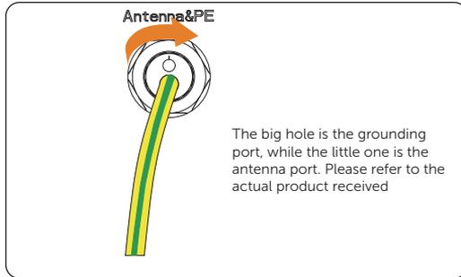
Figure 7-116 Tighting the waterproof connector
