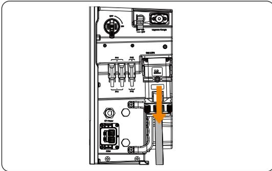
Figure 12-12 Unplugging the AC connector
