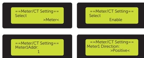
Figure 14-9 Setting meter for the inverter
