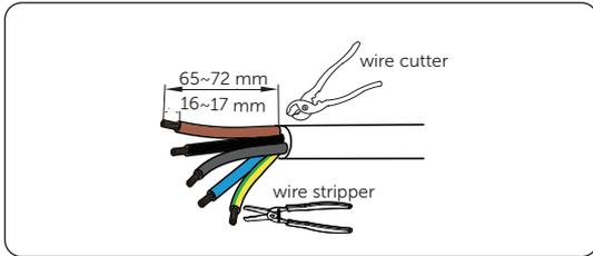
Figure 7-20 Stripping the Grid and EPS cables
