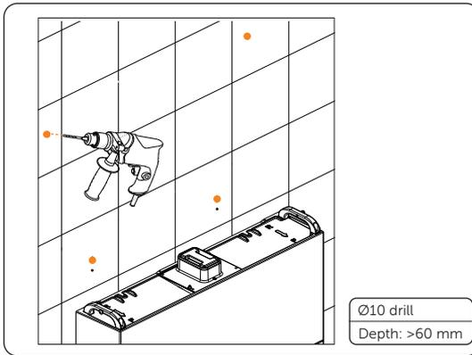
Figure 6-44 Drilling holes
