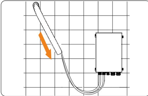
Figure 7-111 Inserting EPS and Grid cables into the corrugated pipe
