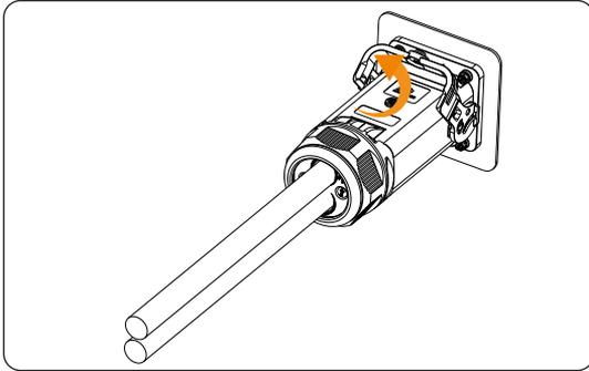
Figure 12-11 Removing the latch of the AC connector
