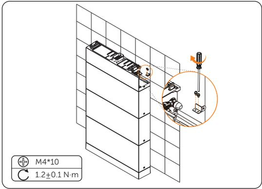
Figure 6-24 Install the anti-tamper bracket
