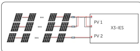
Figure 7-33 "Multi" mode connection diagram for general version
