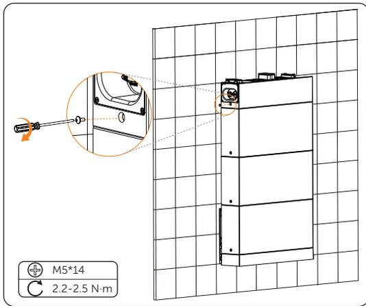
Figure 6-48 Tightening M5 screws
