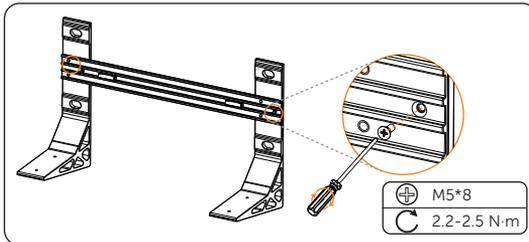
Figure 6-32 Attaching base support and transverse plate
