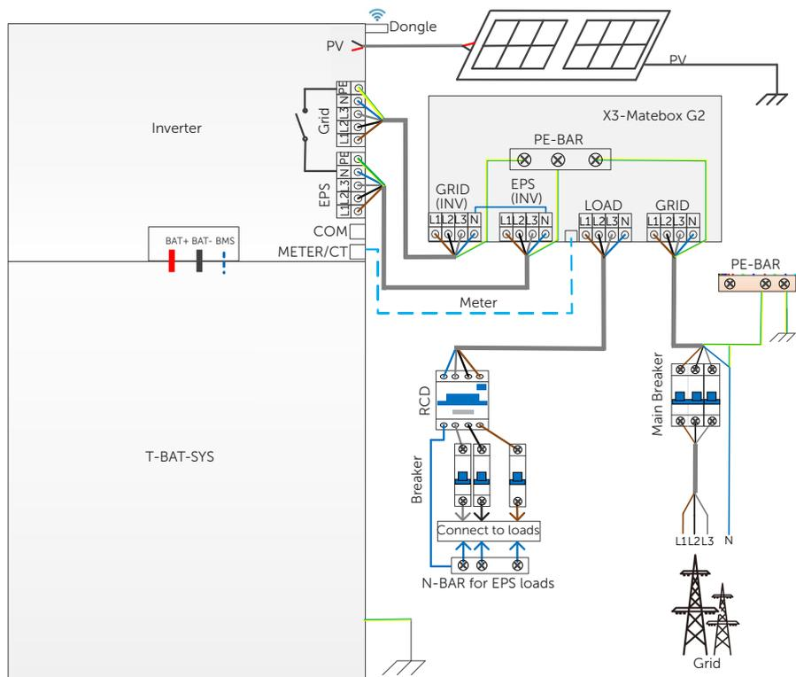
Figure 2-28 System diagram with X3-Matebox G2 for Australia
