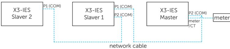
Figure 7-50 Parallel connection without SolaX X3-PBOX device
