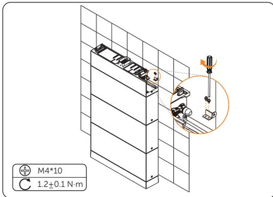
Figure 6-49 Install the anti-tamper bracket
