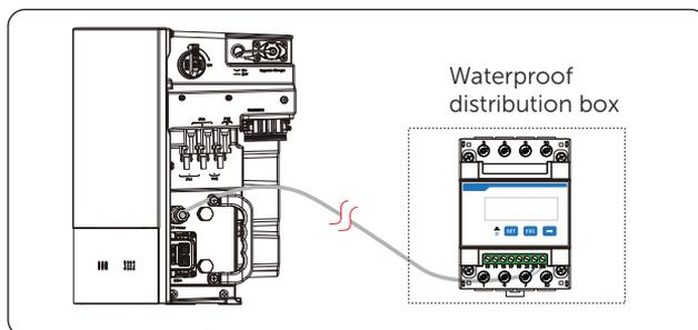
Figure 14-8 Connecting inverter to meter
