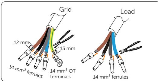
Figure 7-126 Assembling the Grid and Load cable
