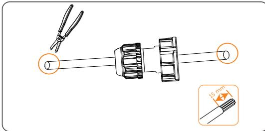
Figure 7-65 Stripping the communication cable for CT
