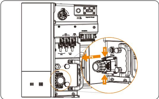
Figure 12-14 Disconnecting the communication connector
