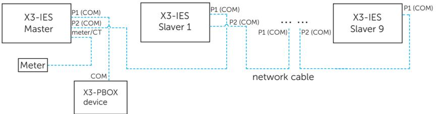
Figure 7-49 Parallel connection with SolaX X3-PBOX device
