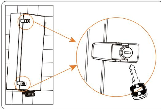
Figure 7-86 Unlocking the buckles
