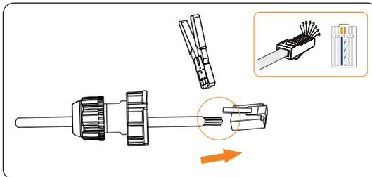
Figure 7-68 Crimping the communication cable for meter
