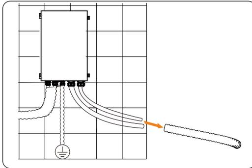
Figure 7-134 Inserting meter cable into the corrugated pipe
