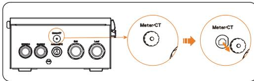
Figure 7-120 Removing the cap
