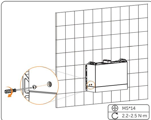
Figure 6-38 Tightening screws
