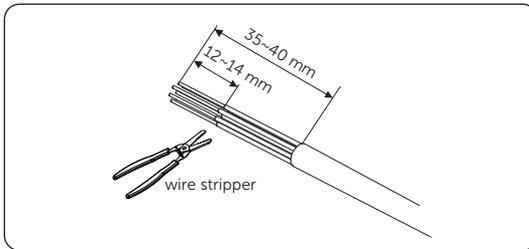
Figure 7-58 Stripping cables
