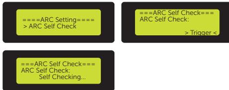
Figure 9-101 Triggering ARC Self Check
