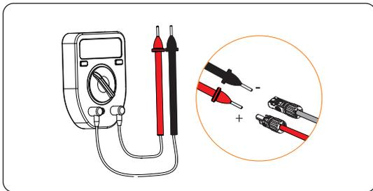
Figure 7-42 Measuring the voltage of PV connectors
