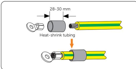
Figure 7-16 Inserting the stripped section into OT terminal
