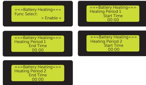
Figure 9-88 Enabling battery heating and setting working periods
