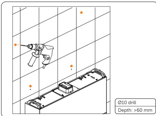
Figure 6-19 Drilling holes
