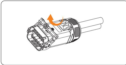
Figure 7-29 Pulling up the latch
