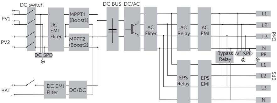
Figure 2-23 X3-IES system circuit diagram
