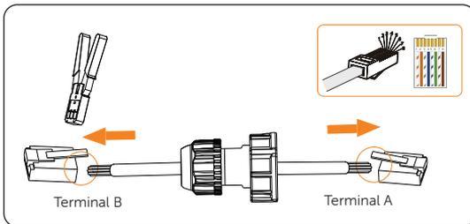
Figure 7-66 Crimping the communication cable for CT
