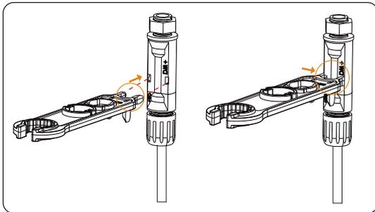
Figure 12-6 Inserting the tool into the PV connector
