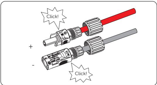
Figure 7-40 Securing PV cables
