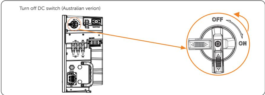
Figure 8-7 Turning off DC switch
