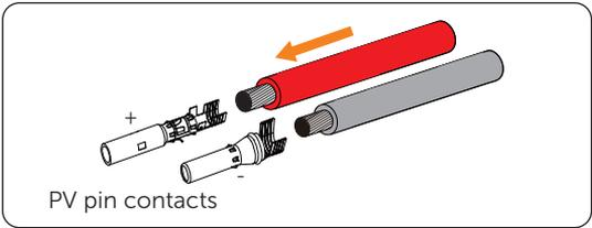
Figure 7-37 Inserting PV pin contacts into PV cables
