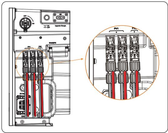
Figure 7-35 Well connected PV cables
