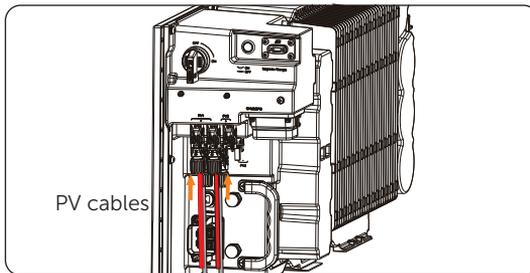
Figure 7-44 Connecting PV cables
