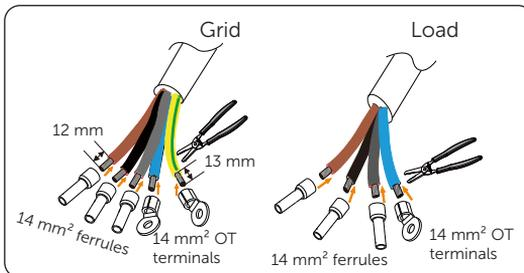
Figure 7-130 Assembling the Grid and Load cable
