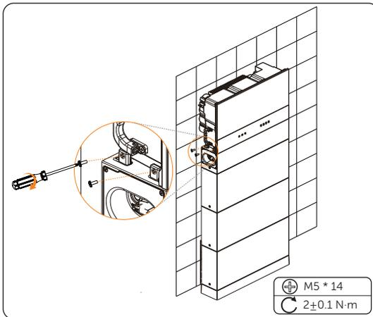
Figure 6-27 Locking the inverter with the BMS
