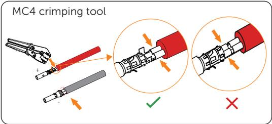
Figure 7-38 Crimping cables with PV pin contacts
