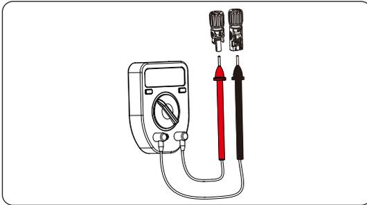
Figure 12-9 Measuring the voltage of PV connectors
