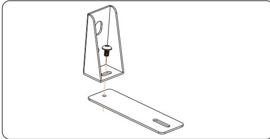
Figure 6-7 Attaching two brackets
