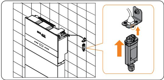
Figure 7-84 Plugging the dongle
