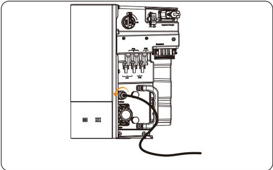
Figure 12-15 Disconnecting the CT/Meter cable
