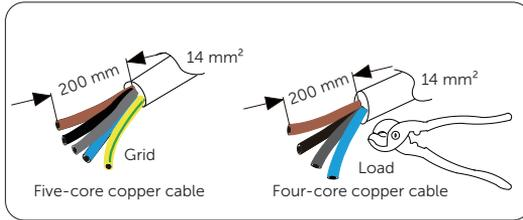
Figure 7-125 Stripping the Grid and Load cable
