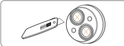
Figure 7-23 Cutting the membrane inside the holes
