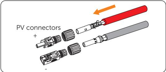
Figure 7-39 Threading PV cables with PV pin contacts connected
