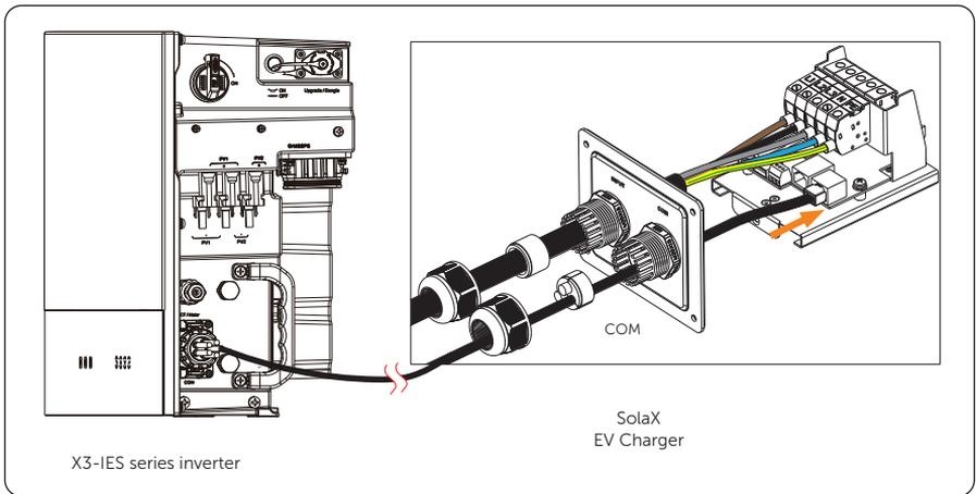
Figure 7-52 Inverter connected with a SolaX EV Charger
