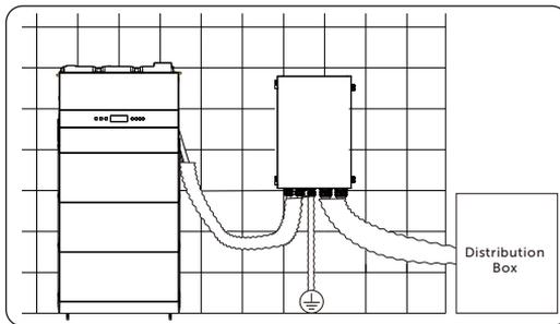
Figure 7-135 Connecting the Grid and Load cables
