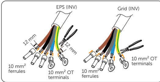
Figure 7-107 Stripping cables and inserting terminals into cables
