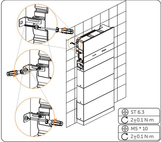
Figure 6-28 Locking the inverter brackets
