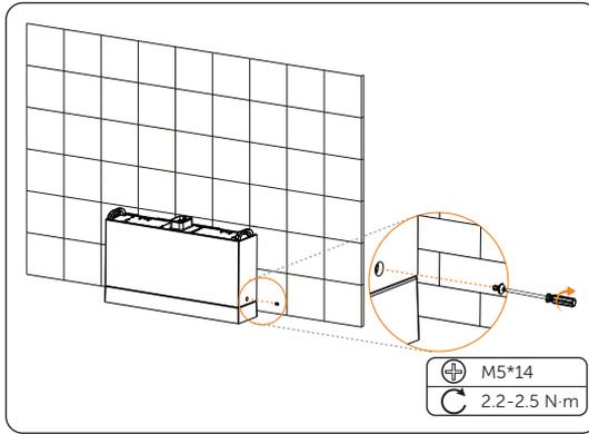
Figure 6-13 Tightening screws
