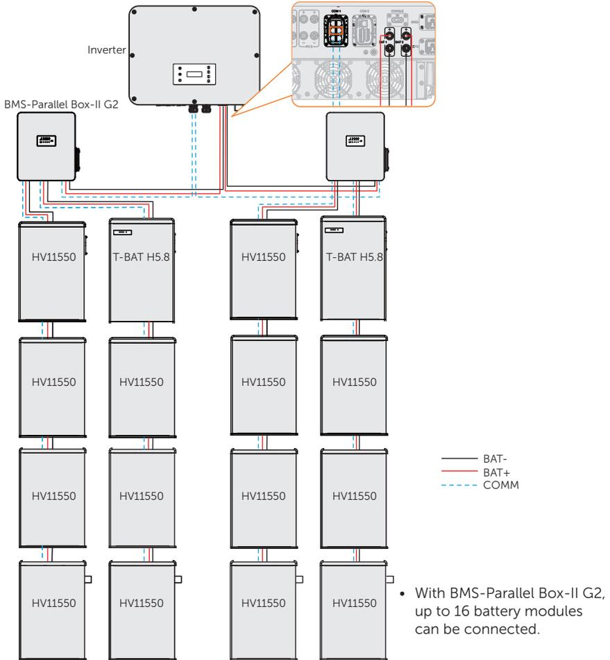
Figure 8-25 Battery connection with BMS-Parallel Box-II G2
